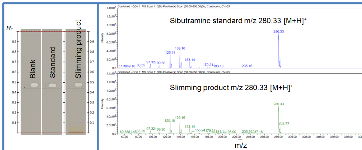
Fig. 2 HPTLC-MS spectra of sibutramine (standard), and sibutramine (slimming product), displayed range m/z 50 to 400
