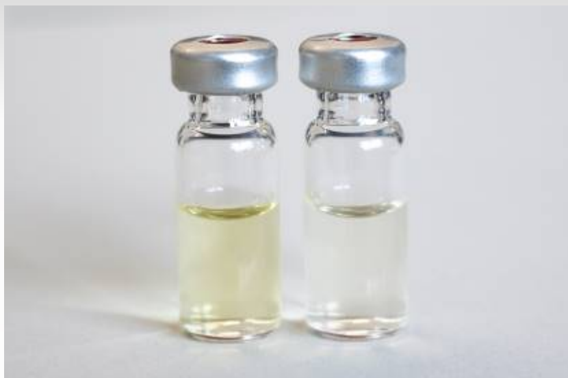
Figure 19: Pistachio (low coloured matrix) - left not cleaned crude extract, right purified with CrossTOX® column
