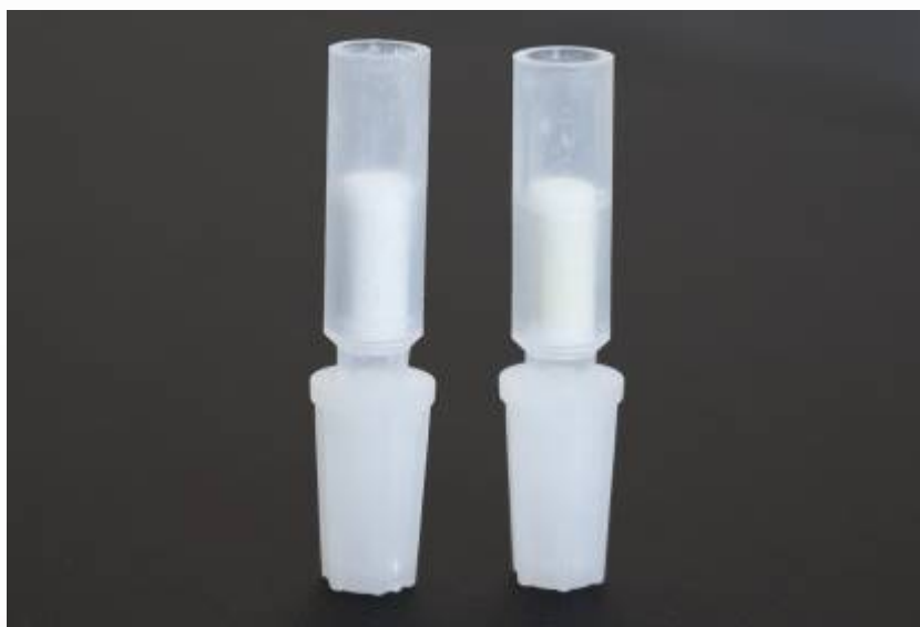
Figure 20: Pistachio (low coloured matrix) - left unused CrossTOX® column, right used CrossTOX® column to clean-up the extract
