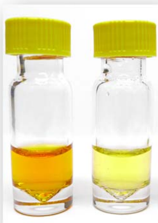
Figure 5: Crude (left) and cleaned extract (right) of bell pepper for UV-VIS measurement
